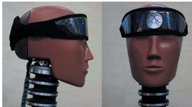
**Figure 4** Head Blast headgear on Hybrid III.
